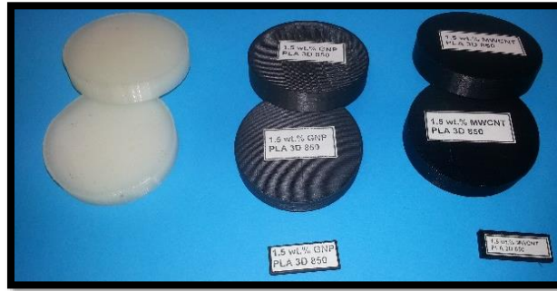
Figure 2. Some samples for thermal measurement produced with FDM technique.
